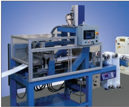
Liquid Filter Bag Machine produces a wide range of products for varying filtration needs, including needle punch and spunbound/meltblown filter media.
