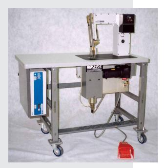
Chase Machine's FS-180 Inverted Ultrasonic Fabric Sealing System "sews" and/or slits knitted, woven, and nonwoven man-made thermoplastic materials without needle or thread. The system differs from Chase Machine's FS-90 in that the welding head is located beneath the table surface, giving the operator greater visibility of the sealed area.
